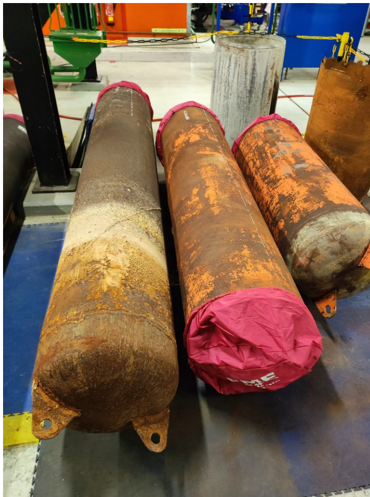
Figure 2-2: Extracted Preheater siphon (inner and outer tubing).
